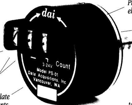
*Precision-machined aluminum baseplate eliminates stripping of hose fitting threads.*
