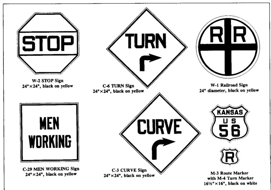
**Figure 3. Signs from the 1927 AASHO rural signing manual. Note the symbols in the "turn" and "curve" signs have a similar appearance. An R or L in a smaller shield below the highway shield was used as an advance turn marker at intersections.<sup>5</sup>**
