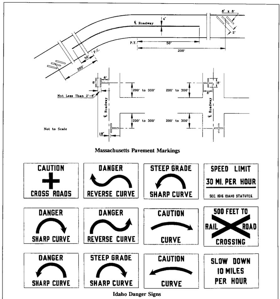
Figure 2. Traffic control devices in the early 1920s.<sup>4</sup>
